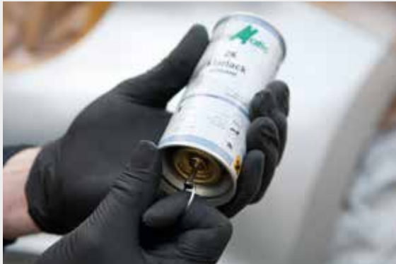
4. Pull hard and twist once by 360°. The blade on the inside cuts the cartridge open.
