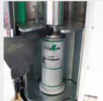
12. Push the can and fitted cylinder back as far as they will go
