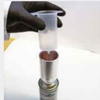
4. Insert the CleanJector into the cylinder
