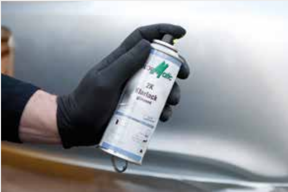
5. After shaking vigorously, the 2K spray is ready to use.
