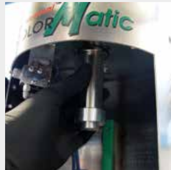
11. Fit the piston and piston rod
