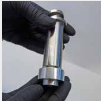
10. Replace the teflon piston with the metal piston
