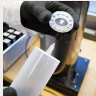
3. Remove the CleanJector's cap
