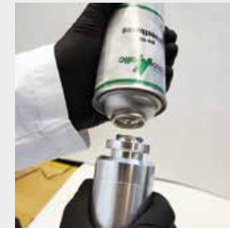
15. Separate the can and cylinder
