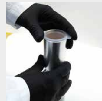
5. Press the CleanJector firmly into place
